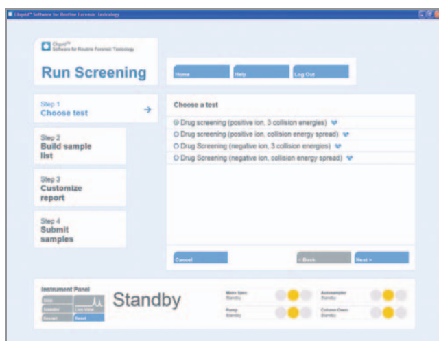
Figure 2: User interface of Applied Biosystems/MDS SCIEX's Cliquant™ Drug Screen and Quant Software for Routine Forensic Toxicology with four-step work flow, 1,200 compound library, new enhanced library search algorithm with automatic library search and reporting function, plus customizable pre-configured report templates.
