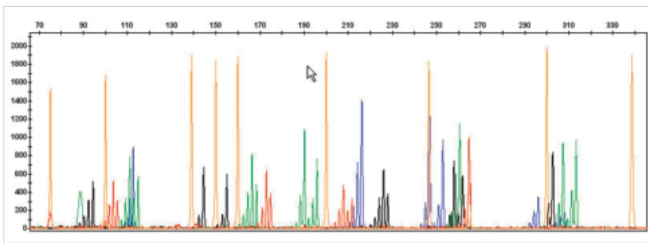
**Figure 3.** Five dye chemistry increases the number of markers that can be run together in a single capillary, thus maximizing throughput. Above is an example of eighteen microsatellite loci co-electrophoresed in a single capillary.
